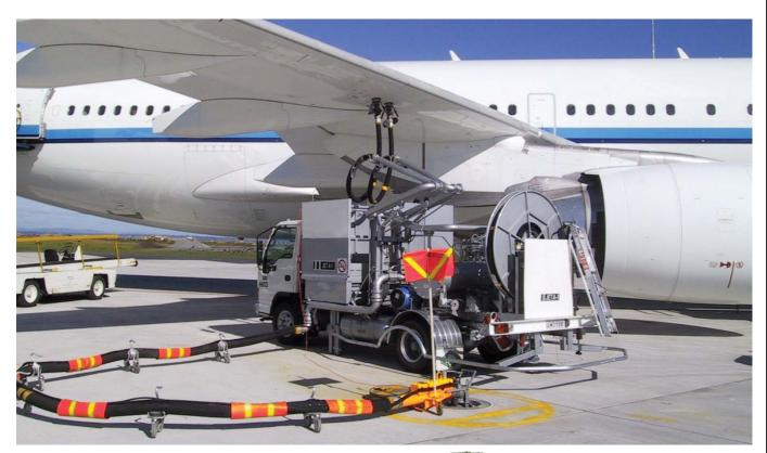
The new "Crocodile" is an input coupler lifting device designed to effortlessly raise and lower the input coupler into position onto the hydrant pit valve.
